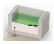
A Styrofoam box with dry ice provides < 1 inch of working height below -50°C for 2 hours
