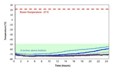
Temperature profile of BioT™ ULT Transporter loaded with dry ice and with lid closed. The entire 8 inch working depth of the transporter remains below -50°C (green shading) for over 24 hours with one charge of dry ice and with the lid closed. Temperature readings were taken every 2 inches above the chamber floor for 8 hours. Inches above base chamber floor: 0 inches (dark purple), 2 inches (purple), 4 inches (lavender), 6 inches (dark blue), 8 inches (light blue).
