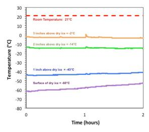
Styrofoam box with dry ice is 14°C at 5.0 cm (2 in) above dry ice
