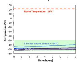
Temperature profile of BioT™ ULT Transporter loaded with dry ice and with lid open. The entire 8 inch working depth of the transporter remains below -50°C (green shading) for over 8 hours with one charge of dry ice and with the lid open. Temperature readings were taken every 2 inches above the chamber floor for 8 hours. Inches above base chamber floor: o inches (dark purple), 2 inches (purple), 4 inches (lavender), 6 inches (dark blue), 8 inches (light blue).
