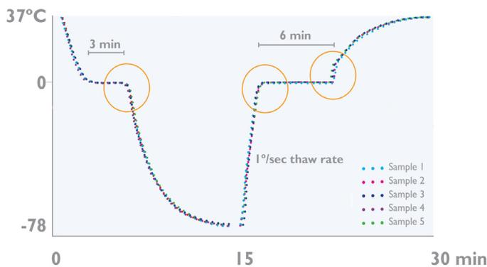
Five consecutive freeze/thaw cycles using a CoolRack CF45 module shows highly reproducible thermal profiles.
